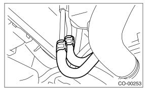
10) Disconnect the radiator outlet hose from thermostat cover.
