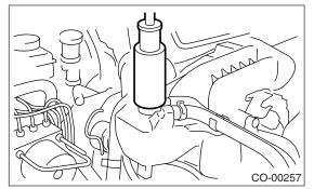
2) Apply a pressure of 122 kPa (1.2 kg/cm<sup>2</sup>, 18 psi) to the radiator to check if:
