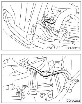
9) Disconnect the ATF cooler hoses from ATF pipes.
