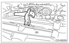
17) Disconnect the two coolant filler tank hoses from radiator.
