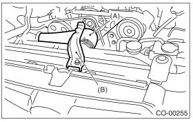
7) Install the reservoir tank. <Ref. to CO(H4DOTC)-30, INSTALLATION, Reservoir Tank.>
