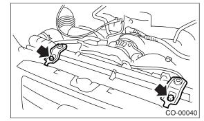
4) Connect the two coolant filler tank hoses to radiator.
