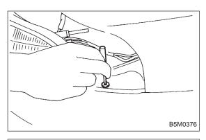
8) Remove clips from both sides of front bumper.
