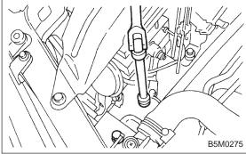
9) Remove bolts (engine compartment side) from bumper stays.
