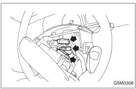
5) Disconnect airbag and horn connectors on back of airbag module. <Ref. to [M2-6].>
