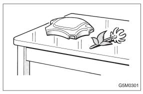
• After removal, the airbag module (driver side and passenger side) should be kept away from heat and light sources, and stored on a clean, flat surface to prevent from any damage to its lower structure.
