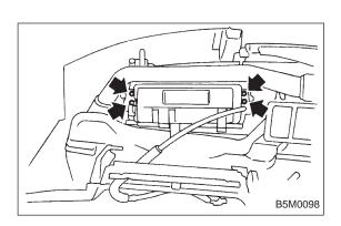
2) Remove four bolts and then carefully remove airbag module.
