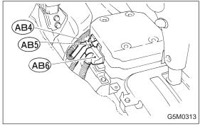
4) Remove console box. <Ref. to 5-4 [W1A0].> Disconnect 12-pin yellow connector (AB6) from airbag control module. <Ref. to 5-5 [M2-6].>
