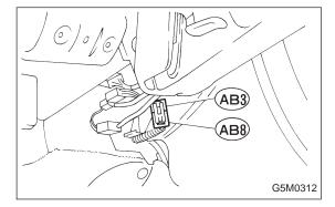
3) Remove lower cover. <Ref. to 5-4 [W1A0].> Disconnect airbag connector (AB3) and (AB8) below steering column.
