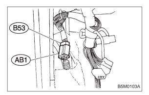
5) Disconnect body harness connector (B53) from connector (AB1).
