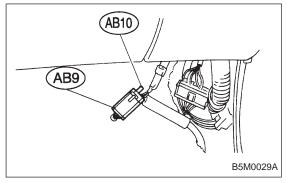
6) Remove front side sill cover and then disconnect airbag connector (AB9) and (AB10). <Ref. to 5-5 [M2-6].>
