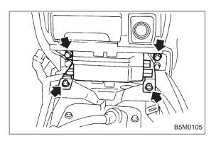
6) Using TORX® BIT T40 (Tamper resistant type), remove two TORX® bolts.
