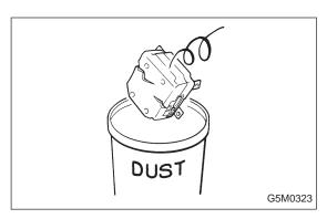
• If the airbag control module is deformed, or if water damage is suspected, replace the airbag control module with a new genuine part.
