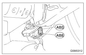
3) Remove lower cover. <Ref. to 5-4 [W1A0].> Disconnect airbag connector (AB3) and (AB8) below steering column. **CAUTION:**
