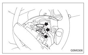
6) Disconnect airbag connector and horn connector on back of airbag module. Remove airbag module, and place it with pad side facing upward. <Ref. to 5-5 [W300].>
