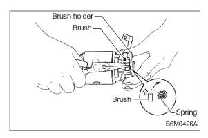
6) Remove brush by lifting up positive (+) side brush spring using long-nose pliers.
