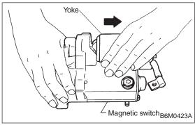
3) Remove yoke from magnetic switch.
