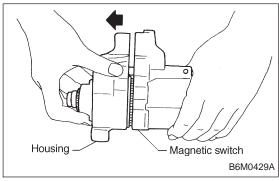
9) Remove housing from magnetic switch.
