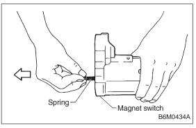
14) Remove coil spring from magnetic switch.
