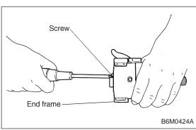
4) Remove screws securing end frame to brush holder.
