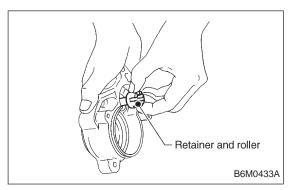
13) Remove retainer and roller from housing.
