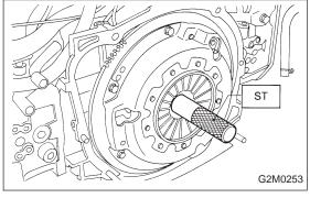
3) Insert ST into the clutch disc and install them on the flywheel by inserting the ST end into the pilot bearing.
