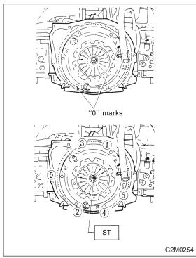
4) Install clutch cover on flywheel and tighten bolts to the specified torque.
