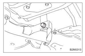
6) Remove front exhaust pipe and center exhaust pipe from hanger bracket.
