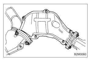
7) Separate front catalytic converter from front exhaust pipe and center exhaust pipe.
