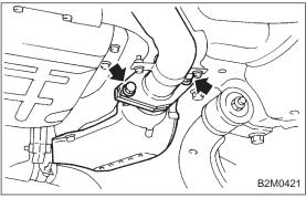
2) Install center exhaust pipe to front catalytic converter.
