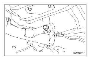
5) Tighten bolt which holds center exhaust pipe to hanger bracket.
