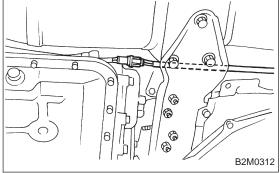
5) Connect rear oxygen sensor connector.
