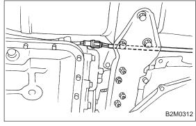
6) Connect rear oxygen sensor connector.
