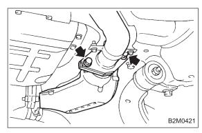
4) Separate center exhaust pipe and rear catalytic converter assembly from front catalytic converter.
