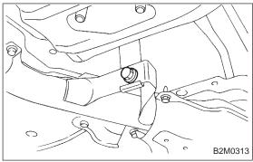
5) Remove center exhaust pipe and rear catalytic converter assembly from hanger bracket.
