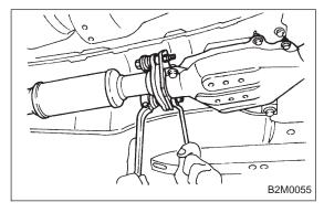
3) Install center exhaust pipe to rear exhaust pipe.
