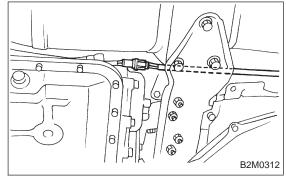
5) Connect rear oxygen sensor connector.
