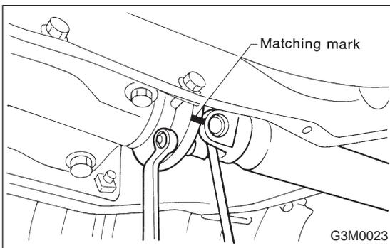
15) Remove propeller shaft. (AWD model)
