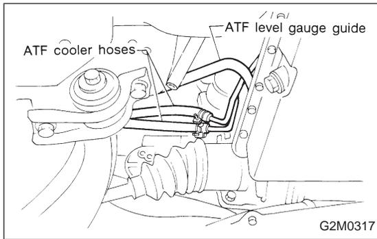
13) Install ATF level gauge guide, and ATF cooler hoses onto pipe. (AT model)
