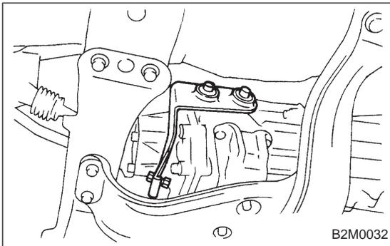
(9) Remove hanger bracket from right side of transmission. (AWD model)
