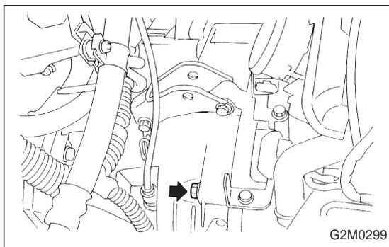
11) Remove bolt which holds right upper side of transmission to engine.
