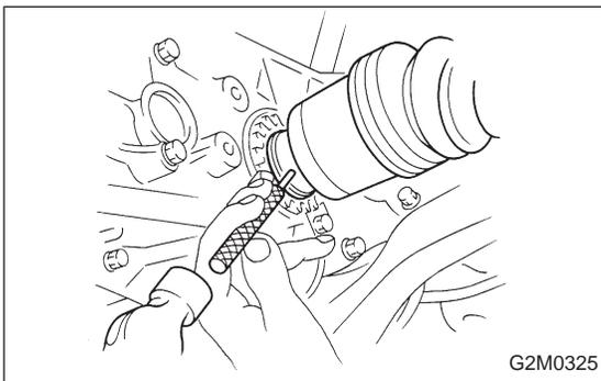
(3) Remove spring pins and separate front drive shafts from each side of the transmission.
