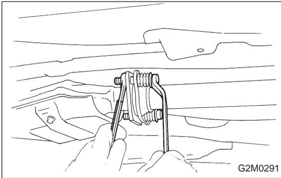
(4) Separate center exhaust pipe from rear exhaust pipe.
