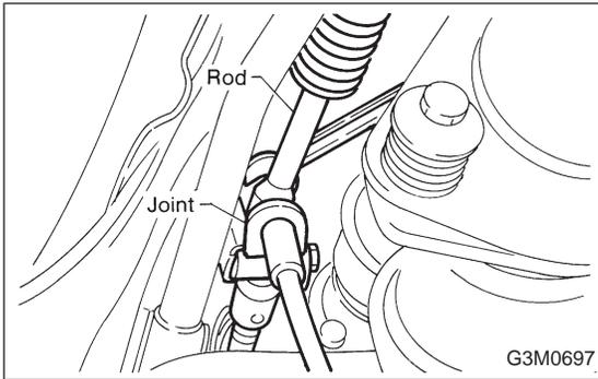
16) Remove gear shift rod and stay from transmission. (MT model)
