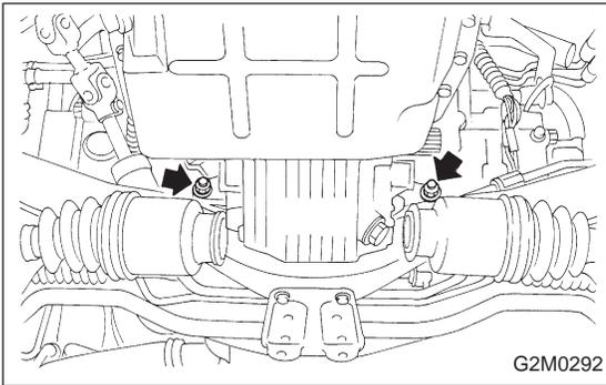
20) Remove nuts which hold lower side of transmission to engine.
