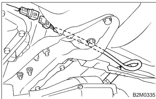
(3) Disconnect connector from rear oxygen sensor.
