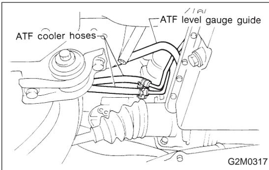
14) Disconnect ATF cooler hoses from pipes of transmission side, and remove ATF level gauge guide. (AT model)
