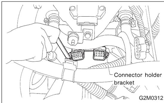
16) Install transmission connector holder bracket.
