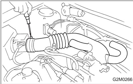
20) Install air intake duct.
