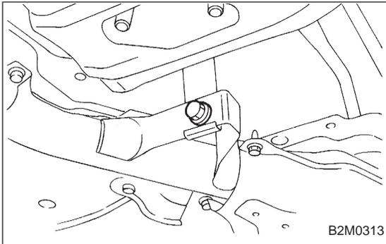
(5) Remove bolt which installs center exhaust pipe to hanger bracket.
