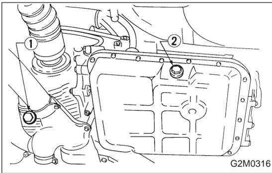
13) Drain ATF to remove ATF drain plug. (AT model)
