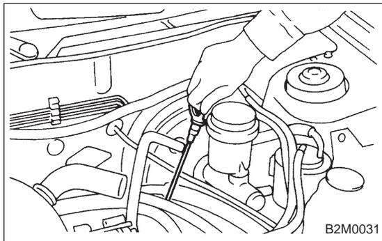
17) Install ATF level gauge. (AT model)
