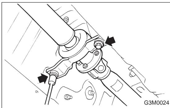
(3) Install center bearing bracket on body.
