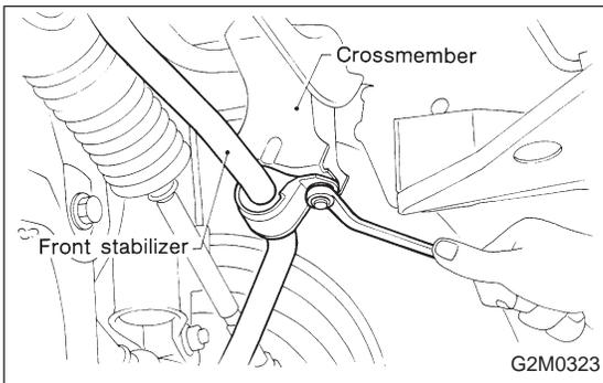
18) Remove bolts which install stabilizer clamps onto crossmember.
