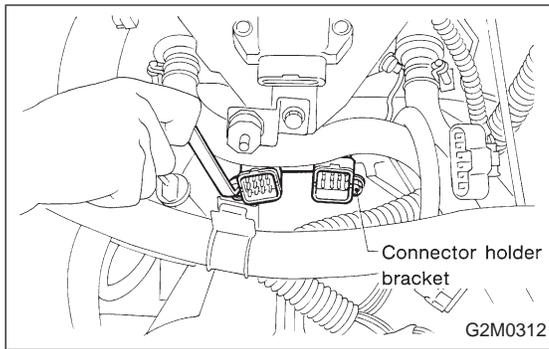
9) Remove transmission connector holder bracket.
