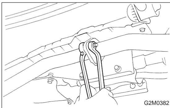
(2) Install rear exhaust pipe to muffler. (AWD model)
