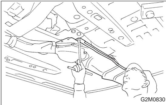
(8) Remove heat shield cover of rear exhaust pipe. (AWD model)
