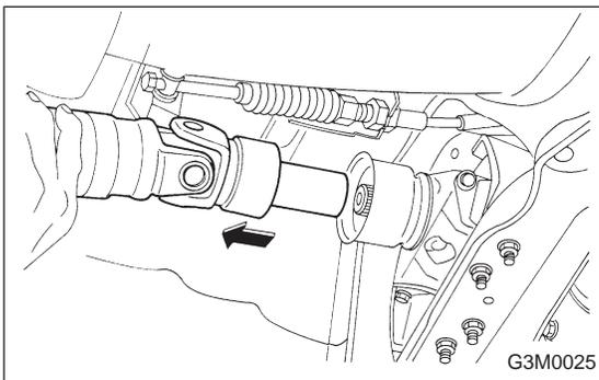
(4) Remove propeller shaft from transmission.
