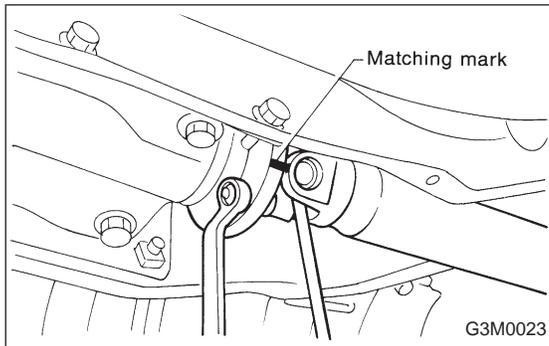
14) Install propeller shaft. (AWD model)
