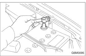
8) Connect ground cable to battery terminal.
