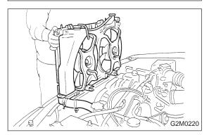
2) Install radiator while fitting radiator pins to cushions.
