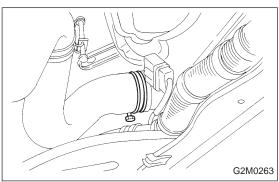
7) Disconnect connectors of radiator main fan and sub fan motor.
