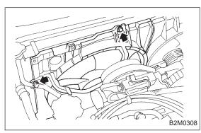
4) Remove four bolts holding shroud to radiator.
