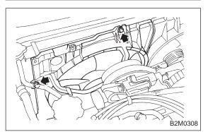
4) Remove four bolts holding shroud to radiator.
