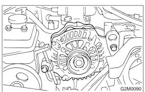
3) Install generator on bracket and temporary tighten installing bolts.
