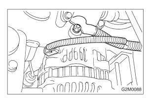
6) Connect connector and terminal to generator.
