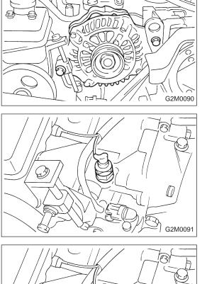
(4) Remove bolts which install generator on bracket.
