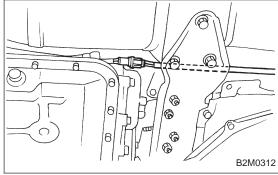
6) Connect rear oxygen sensor connector.
