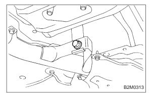
6) Remove front exhaust pipe and center exhaust pipe from hanger bracket.
