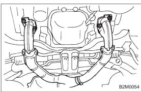
5) Remove bolts which hold front exhaust pipe onto cylinder heads.
