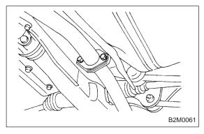
2) Separate rear exhaust pipe from muffler.
