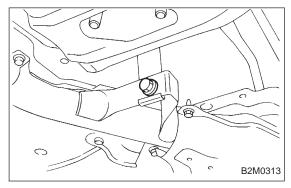
2) Install front exhaust pipe and center exhaust pipe. And temporarily tighten bolt which installs center exhaust pipe to hanger bracket.
