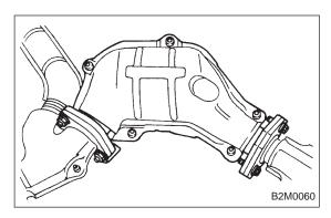
7) Separate front exhaust pipe from front catalytic converter.
