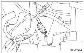
2) Disconnect connector from front oxygen sensor.
