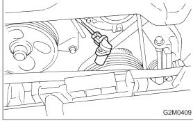
2) Remove crankshaft position sensor, and disconnect connector from it.
