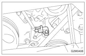
3) Installation is in the reverse order of removal. *Tightening torque:*6.4±0.5 N·m (0.65±0.05 kg-m, 4.7±0.4 ft-lb)
