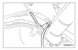
5) Remove front oxygen sensor.
