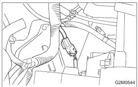
2) Disconnect connector from front oxygen sensor.
