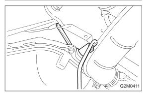
Install front oxygen sensor.
