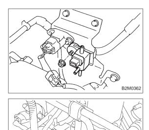
3) Remove pressure sources switching solenoid valve from bracket.
