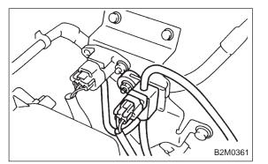
9) Check duty ratio of idle air control solenoid valve with Subaru Select Monitor.
