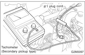
5) Check idle speed when unloaded. (With headlights, heater fan, rear defroster, radiator fan, air conditioning, etc. OFF)
