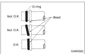
Visually inspect the O-ring surface, the O-ring mating surface, the threads and the connection points. If a defective part is found, replace it.
