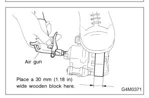
3) Gradually supply compressed air via inlet of caliper body to force piston out.
