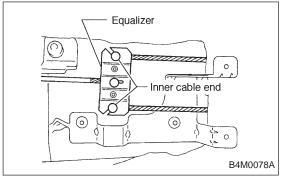
7) Remove inner cable end from equalizer.
