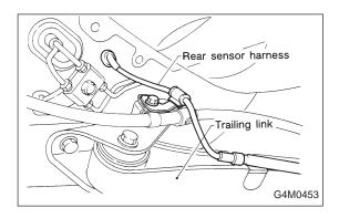
4) Install rear sensor harness on rear trailing link.
