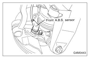
4) Remove bolts which secure front ABS sensor to housing, and remove front ABS sensor.
