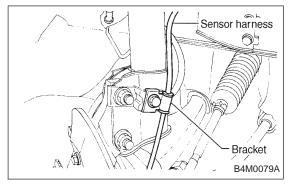
2) Remove bolts which secure sensor harness to strut.
