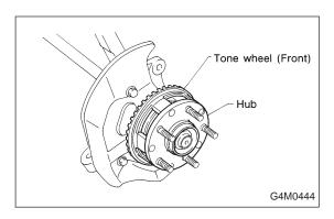
7) Remove tone wheel while removing hub from housing and hub assembly. <Ref. to 4-2 [W1B0].>
