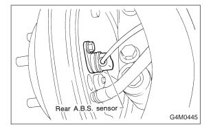
2) Temporarily install rear ABS sensor on back plate.
