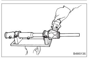
2) Install packing on valve assembly. Insert valve assembly into place while facing rack teeth toward pinion. **CAUTION:**
