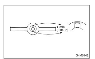
Rack ASSY Rack stopper G4M0143 NOTE: If ST is used, grind area (shown in figure) by 1 mm (0.04 in) in advance. ST 926340000 WRENCH
