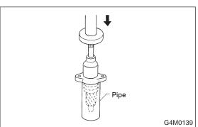
3) Draw out pinion and valve assembly from valve housing, as necessary, using pipe of I.D. 44 to 46 mm (1.73
