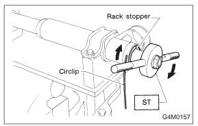
4) Insert rack assembly into rack housing from cylinder side, and remove ST after it has passed completely through oil seal.
