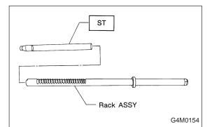
2) Fit ST over toothed portion of rack assembly, and check for binding or unsmooth insertion. If any deformation is noted on flats at the end of rack, shape by using file, and wash with cleaning fluid.
