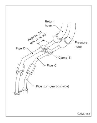
3) Temporarily connect pipes C and D to pipes (on the gearbox side).
