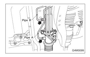
7) Connect pipes A and B to four pipe joints of gearbox. Connect upper pipe B first, and lower pipe A second.
