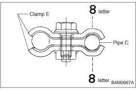
4) Temporarily install clamp E on pipes C and D.
