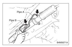
7) Connect pipes A and B to four pipe joints of gearbox. Connect upper pipe A first, and lower pipe B second.
