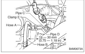
3) Temporarily connect pipes C and D to control valve of gearbox.
