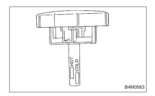
(1) Check at temperature  $21^{\circ}C$  (70°F) on reservoir surface of oil pump.
