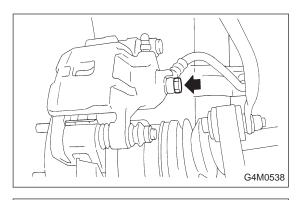
7) Models equipped with rear disc brakes:Remove union bolt from brake caliper.8) Models equipped with rear drum brakes:Disconnect brake hose from brake pipe from strut, and
