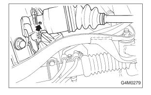
5) Remove spring pin which secures transmission spindle to DOJ.
