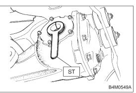
2) Using ST, install DOJ into differential.ST 28099PA090 SIDE OIL SEAL PROTECTOR
