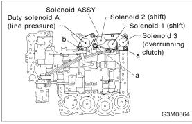
(2) Install solenoid valves. Shift solenoids, 1, 2 and 3, and duty solenoid A (line pressure).
