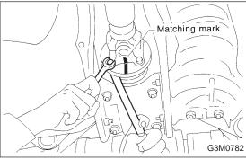
(4) Remove propeller shaft.
