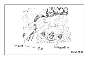
(3) Install valve body and two brackets.
