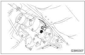
(3) Install vehicle speed sensor 1.
