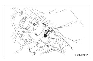
(6) Remove vehicle speed sensor 1.
