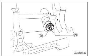
9) Remove outer snap ring (20) and pull out speedometer driven gear (1). Next, remove vehicle speed sensor 2, oil seal, speedometer shaft 22 and washer.
