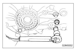
9) Position balls ①, checking ball springs ③ and gaskets ① into 3-4 and 1-2 rod holes, and install plugs ②.
