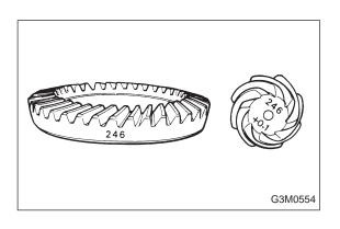
1) Alignment marks/numbers on hypoid gear set ① The upper number on driven pinion is the match number for combining it with hypoid driven gear. The lower number is for shim adjustment. If no lower number is shown, the value is zero. The number on hypoid driven gear indicates a number for combination with drive pinion.
