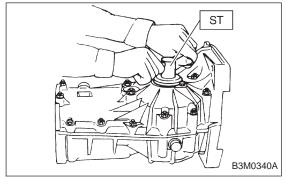
(3) Remove weight and screw in retainer without O-ring on the upper side and stop at the point where slight resistance is felt.
