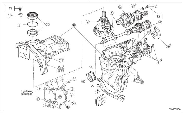
Tightening torque: N·m (kg-m, ft-lb) T1: 25 (2.5, 18) T2: 29±3 (3.0±0.3, 21.7±2.2)
