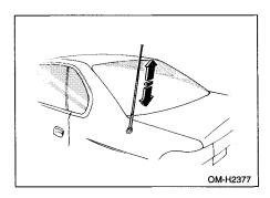
The power antenna automatically extends or retracts when the radio is turned on or off.
