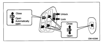
All door windows can be controlled by the main switch at the driver side door.
