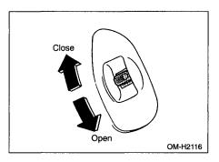
When the lock switch, located on the driver's side door, is in the "LOCK" position, the passengers' windows cannot be operated with the passengers' switches.
