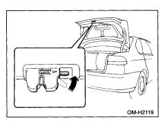
The inside trunk lid release can be cancelled to help prevent unauthorized entry into the trunk. To cancel the trunk lid release, set the lid release cancel lever (located on the inside of the trunk lid, mounted to the trunk lid latch) to the "CANCEL" position. When this lock is in the "CANCEL" position, the trunk can be opened only by the master key.
