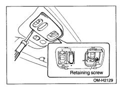
2. Remove the spot light lens by hand, then remove the switch body retaining screw and take off the sunroof switch.
