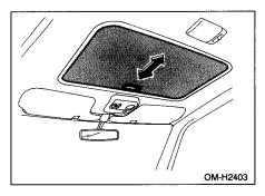
Open and close the sun shade by sliding it forward or backward while the sunroof is fully closed or tilted up.
