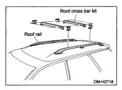
Luggage can be carried on the roof after securing the roof cross bar kit to the roof rail. When installing the roof cross bar kit on the roof rail, follow the manufacturer's instructions. The roof cross bar kit is designed to carry loads (luggage and roof rack) of not more than 100 lb. (45 kg).
