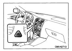
Day or night, if your vehicle becomes a traffic hazard, use the hazard warning flasher. Avoid stopping on the road. It is best to safely pull off the road if a problem occurs. Turn on the hazard warning by pushing the hazard warning flasher switch. Turn it off by pushing the switch again.
