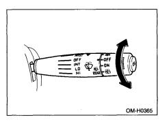
To turn the rear wiper on, turn the end of the wiper control lever to the "ON" position.
