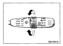
When the wiper switch is in the "INT" position, turn the dial to adjust the operating interval of the wiper.
