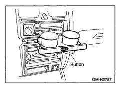
To use the cup holder, push the button and it will automatically pop out then pull it out completely.
