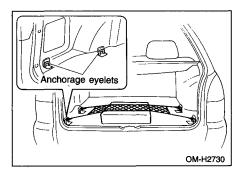
The luggage compartment is equipped with four anchorage eyelets so that luggage can be secured with a luggage net or ropes.
