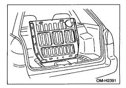
The storage tray is located under the floor of the luggage compartment and can be used to store small items. To open the lid, pull the handle up.
