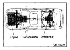
Inspect the following for oil leaks:
