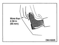
Depress the pedal with a force of approximately 294 N (66 lb, 30 kg) and measure the distance between the upper surface of the pedal pad and the floor.
