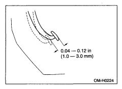
Stop the engine and firmly depress the brake pedal several times. Lightly press the brake pedal down by finger to check the free play with a force of less than 10 N (2 lb, 1 kg).
