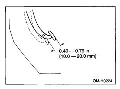
Lightly press the clutch pedal down with your finger until you feel resistance, and check the free play.
