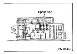
6. If the same fuse blows again, this indicates that its system has a problem. Contact your SUBARU dealer for repair.
