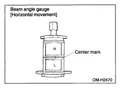
2. Look at the beam angle gauge (horizontal movement). The center mark should not deviate from the line on the outer case by more than two segments on either side of the gauge.
