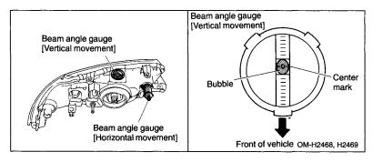
1. Look at the beam angle gauge (vertical movement). The bubble on the gauge should not deviate from the center of the gauge by more than four segments on either side of the gauge.
