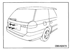
Use M5 x 12 bolts to install a license plate on the rear gate.
